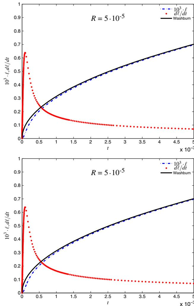
**Figure 3.** Viscous case  $\mu = 5 \text{ mPa} \cdot \text{s}$  with  $R = 0.05$  mm. Top frame: results found by invariance. Bottom frame: direct numerical results. Washburn solution and  $\ell(t)$  are magnified by a factor  $10^3$ .
