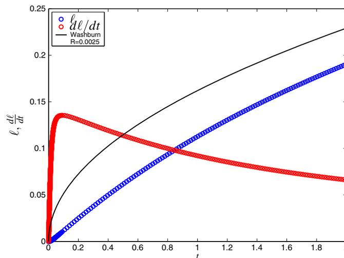
Figure 5. Adaptive step-size results:  $\ell(t)$  and its first derivative. Solution obtained by a direct computation. Viscous case  $\mu = 1 \text{ mPa} \cdot \text{s}$  with  $R = 0.0025 \text{ mm}$ .
