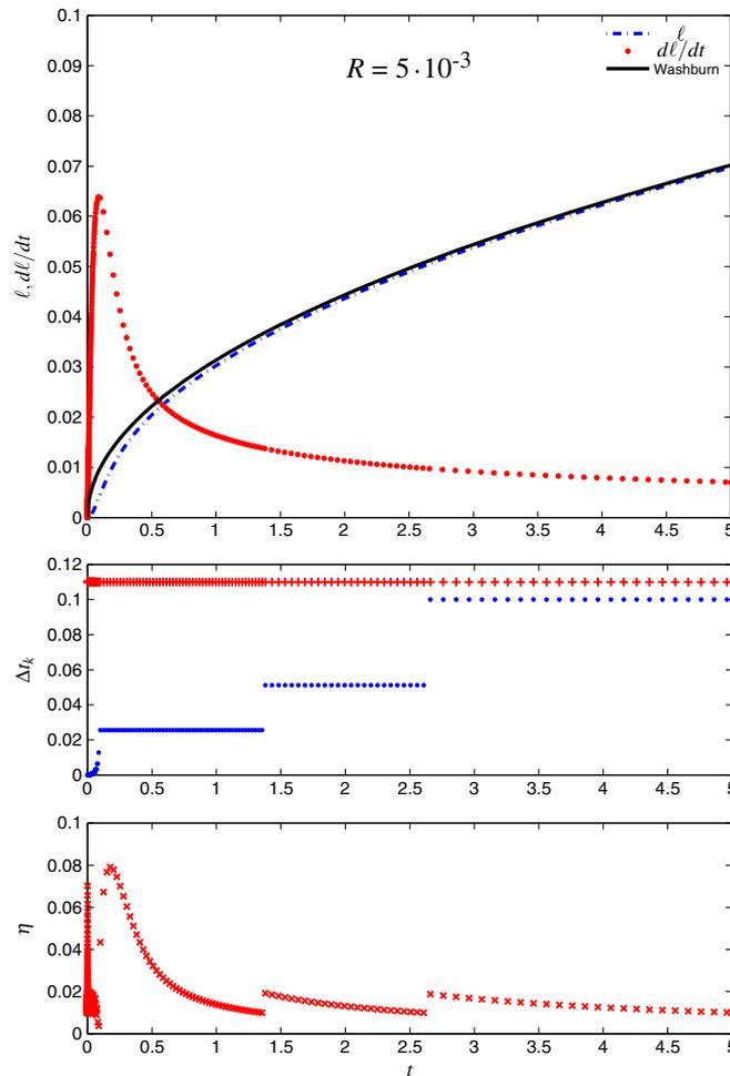
**Figure 2.** Adaptive step-size results. Here, by setting  $R = 5$  mm, we get:  $\lambda = 10^{-2}$ ,  $\mu = 0.5$  mPa · s,  $\rho = 9.18$  Kg/m<sup>3</sup>,  $\gamma = 0.197$  mN/m. From top to bottom: numerical solution, adaptive step-size selection  $\Delta t_k$ , and monitor function  $\eta$ .
